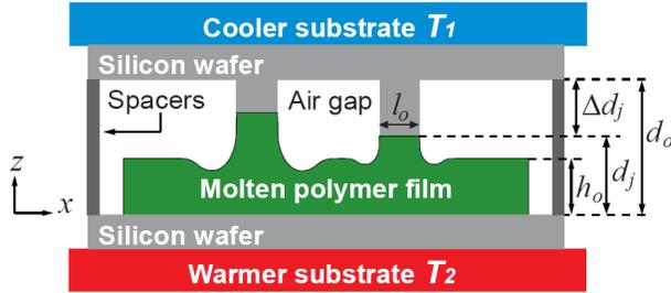
**Figure 1** Schematic diagram of experimental setup for nanopillar formation. Upper wafer contains protruding elements (labeled by index  $j$ ) of diameter  $l_o$  and depth  $d_o - d_j$ . For the numerical simulations of the formation process in this study,  $h_o = 100$  nm,  $d_o = 285$  nm and  $\Delta T = T_2 - T_1 = 170^\circ\text{C} - 124^\circ\text{C} = 46^\circ\text{C}$ . All remaining variables and material properties are given in the text.
