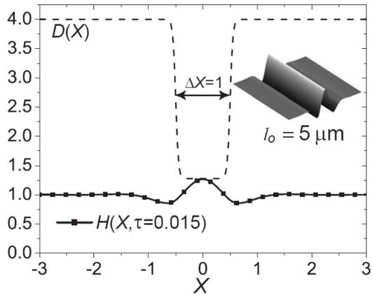
**Figure 4** Film shape  $H(X,\tau)$  induced by a ridge placed in close proximity to the polymer surface. The ridge width  $l_o$  is much smaller than the instability wavelength described by Eq. (2) pertinent to a flat wafer with no protrusions. Remaining parameter values are given in the text.
