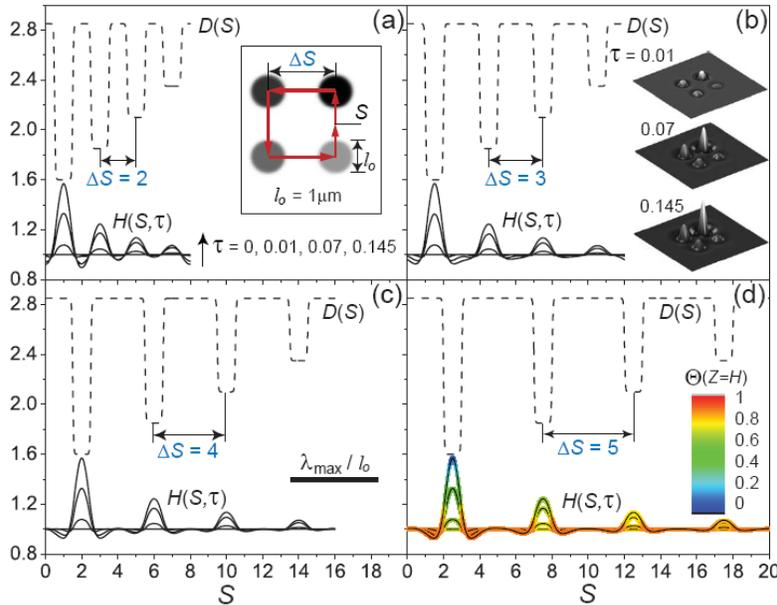
**Figure 2** Plots of the film thickness  $H(S,\tau)$  as a function of perimeter distance  $S$  (measured in counterclockwise fashion) as a function of time  $\tau = 0.0, 0.01, 0.07$  and  $0.145$  for a square array of cylindrical protrusions of diameter  $l_o=1 \mu\text{m}$  and decreasing size 1.25, 1.0, 0.75 and 0.5 (in units of  $h_o$ ), separated by an equal distance (a)  $\Delta S=2$ , (b)  $\Delta S=3$ , (c)  $\Delta S=4$  and (d)  $\Delta S=5$ .
