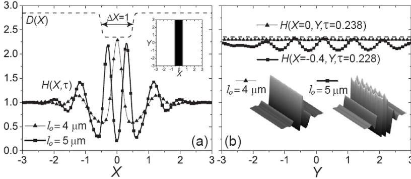
**Figure 3** Plots of film shapes induced by a top wafer patterned with a single extended protrusion resembling a ridge of width 4 or 5  $\mu\text{m}$ . (a) Cross-sectional view of film surfaces along the  $X$ -axis. (b) Cross-sectional view of film surfaces along the  $Y$ -axis. Remaining parameter values are given in the text.
